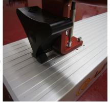
2) Mount one of the lower feet to the appropriate side plate. Use the socket head M6-1x16 screws. There are four screws
