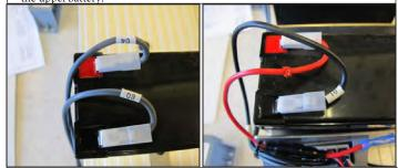
The newly installed batteries should be positioned as shown.
