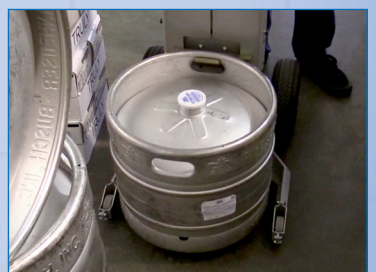
Adjustable lifting bracket accommodates shorter kegs
