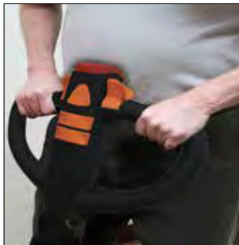
Auto-reversing "belly bump" switch protects operator. Dual lift/lower controls and horn access are all within easy reach.
