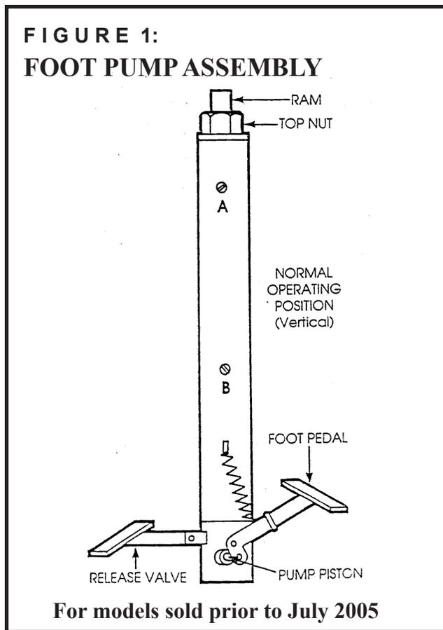
lowered. Remove screw B fig. 1 Oil should be just below this level. If oil is needed use Conoco Super Hydraulic 32. **DO NOT USE BRAKE FLUID.** The hydraulic oil does not have to be changed unless it is unusually dirty (very dark in color) or if water is introduced due to condensation-weekly.
