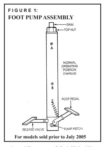
lowered. Remove screw B fig. 1 Oil should be just below this level. If oil is needed use Conoco Super Hydraulic 32. DO NOT USE BRAKE FLUID. The hydraulic oil does not have to be changed unless it is unusually dirty (very dark in color) or if water is introduced due to condensation-weekly.
