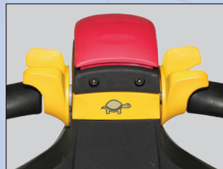
Turtle-speed button reduces drive speed by 50% for precise positioning
