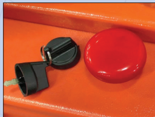
Key switch prevents unauthorized use; Emergency e-stop halts operation
