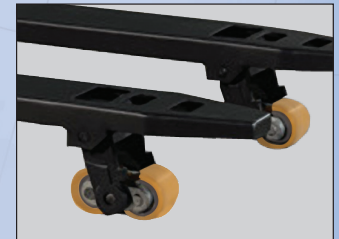
Articulating front casters provide smooth travel on uneven surfaces
