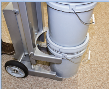
Lifting yoke holds pails in place.
