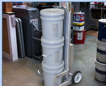
200 lb. lifting capacity safely handles 3 pails at a time.
