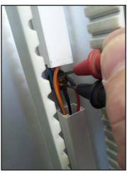
Take off front cover of the mast and locate the back side of charger inlet. Connect the charger. Led # 2 will shortly turn green and then go off. Led #1 will turn red to indicate the charger is in step 1 (Bulk charging). Measure DC voltage on the plug. While charger is at step 1 the voltage shall be increasing slowly reading about 26-29V DC. When charger goes green the voltage will drop below 27,4VDC.
